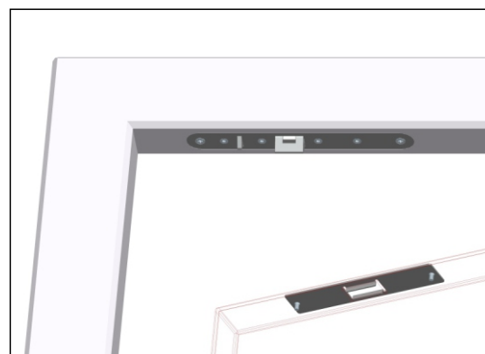
Installation on top
