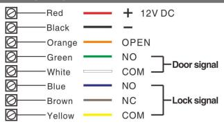
Can not be used directly by power on or power off, must be controlled through OPEN wire to unlock.
