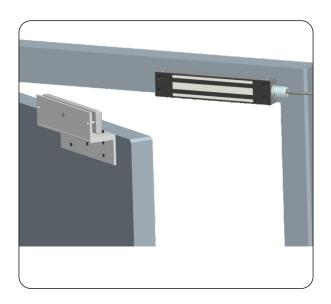
**Step 1:** There must be 2 metal washers and 1 rubber washer between armature plate and Z-shaped bracket. Put the rubber washer between 2 metal washers. Lock the flattop screw in the middle of armature plate to the Z-shaped plate.
